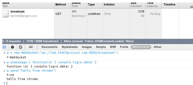
Figure 6. WebSocket connectivity in Chrome Developer Tools' Network panel
