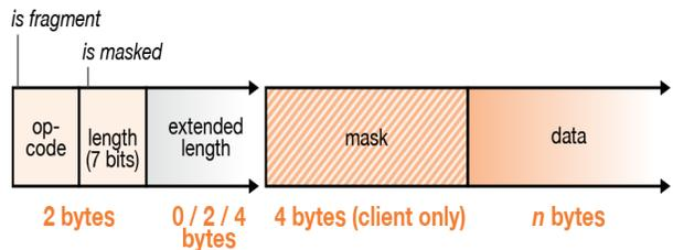
Figure 2. Components of a WebSocket Frame
