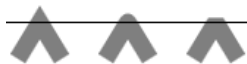
Three paths, each drawn up to the thin black line and back down. From left to right, the lineJoin property of each is "miter", "round", and "bevel".
