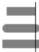
Three gray lines drawn to the thin black line. From top to bottom, the lineCap property of each is "butt", "round", and "square".
