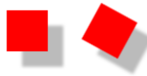
A square drawn with a shadowOffsetX and shadowOffsetY of 15. The shadow is drawn evenly 15 pixels offset in both axes. To the right is the same square drawn with the same shadowOffsetX and Y, but the context was rotated about the square's center.
